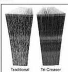
Tech-ni-Fold's "Tri-Creaser" is go to totally eliminate fibre cracking
